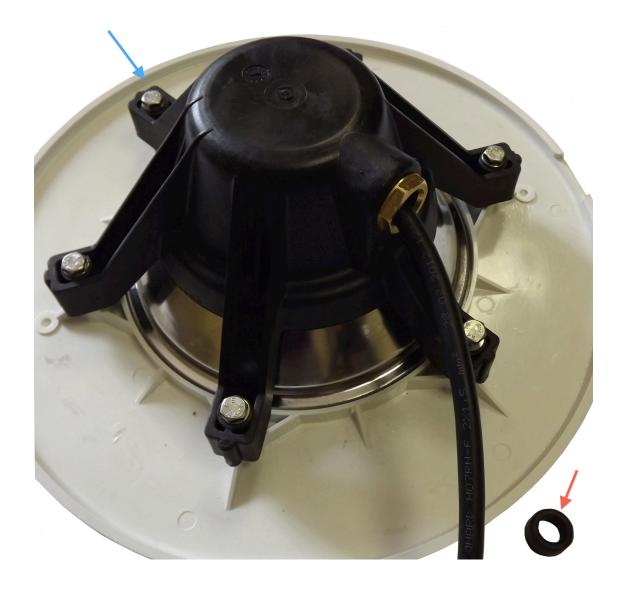
**ATTENTION!** With the PAR56 LED lamp, with its cable already connected to the body, the connection is waterproof and, therefore, the cable gland and/or the gasket indicated by the red arrow **MUST NOT BE** closed or mounted. In this way the water could make the lamp cooler; we advise not to excessively tighten the screws indicated by the blue arrow, as it is likely to deform the lamp's mechanics. Tighten the minimum necessary to maintain the lamp in position.
