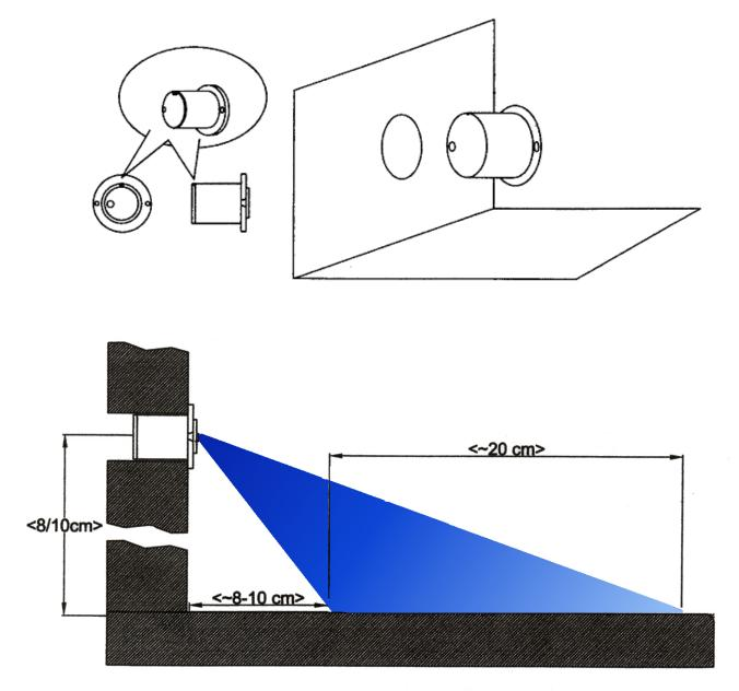
ATTENTION! THE LIGHT BEAM MAY CHANGE ACCORDING TO THE SPOT MODEL AND THE INCORPORATED LENS.
